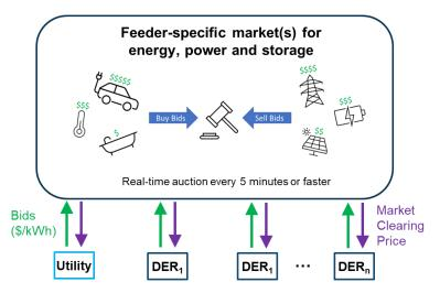
building console. In combination, the DER bids and clearing price determine which DERs consume energy from the grid and which DERs put energy onto the grid during the market interval. Real-time human participation is not required, but building occupants always have the option to override participation or change their previously expressed preference.
